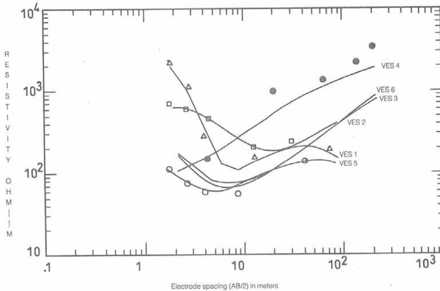
Fig. 5. Six VES curves with electrode spacing (meters) versus apparent resistivity (ohm-m) obtained along a traverse parallel to the trend of Wadi Bishah.
