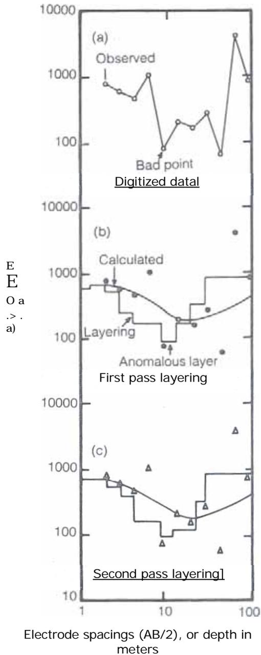
Fig. .6. Automatic interpretation of VES 2: (a) digitized curve, (b) first-pass results with anomalous layer and poorly-fitting calculated curve, and (c) second-pass results with anomalous layer eliminated and calculated curve still not closely matching the observed curve.
