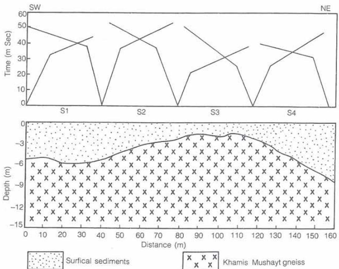
Fig. 7. Geological section and travel-time versus distance plot showing the general relationships of seismic velocities and cross-over distances between four seismic refraction spreads along a SW - NE traverse.
