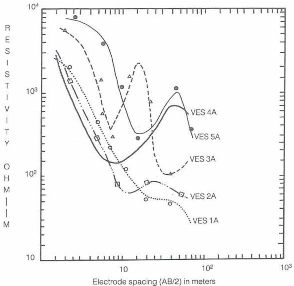
**Fig. 4 Six VES curves with electrode spacing (meters) versus apparent resistivity (ohm-m) obtained along a traverse perpendicular to the trend of wadi Bisleale.**
