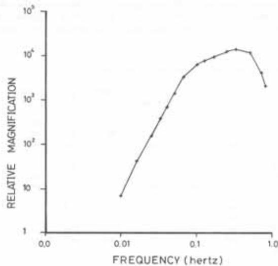
Fig. 2. Analog system response curves for the Dhahran (DHR) station. The intermediate period response curve extends from 0.01 to 0.8 Hz.
